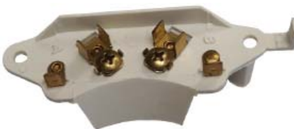
terminal board mounting holes : 3-5/16" C.-C. top : 2 bolts, 6 quick connects bottom : 4 quick connects
