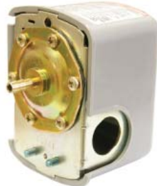
pressure switch 1/4" barb fitting factory set at 30-50 PSI
