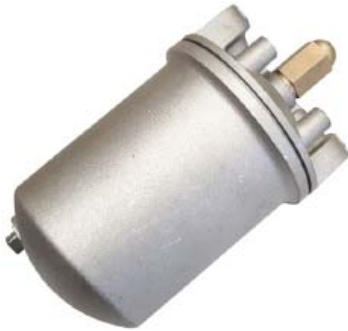
aluminum filter housing port sizes : 3/8", 300psi uses filter CUNO-300 or CUNO-300PT body diameter : 3-1/8" overall size : 3-5/8 x 6-1/2"
