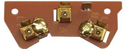
terminal board mounting holes : 2-3/8" C.-C. top : 2 bolts, 8 quick connects bottom : 3 quick connects
