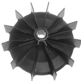
plastic cooling fan, 2 flats on I.D. .660 x 5-5/16"
