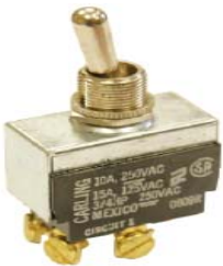
toggle switch screw terminals 3/4hp rating 15A@125V / 10A@250V body : 1-3/8 x 3/4 x 1"
