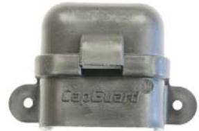
weather proof capacitor guard fits oval capacitors that are 2-1/16" X 1-1/4" mtg. holes : 2-13/16" C.-C.
