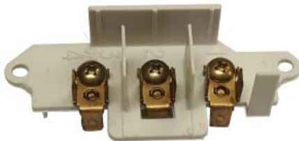
terminal board mounting holes : 3-5/16" C.-C. top : 3 bolts, 6 quick connects bottom : 3 quick connects
