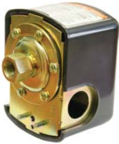
Pressure Switch 1/4" Female Fitting factory set at 30-50 PSI
