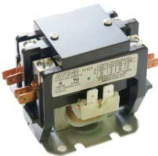
Mars relay #91423 2 pole, 40A, 208/240 VAC
