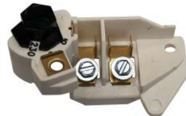
terminal board / voltage change switch dual voltage / 1-speed mounting holes : 2-1/8" C.C. top : 2 bolts, 3 quick connects bottom : 3 quick connects
