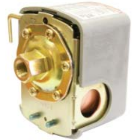
pressure switch low pressure cut-off 1/4" female fitting factory set at 30-50 PSI
