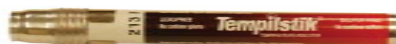
temperature indicator 213F. / 101C. stroke surface. a liquid smear will appear at the rated temperature
